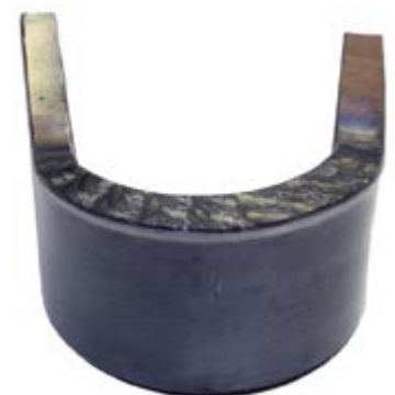
Side Bend: Fully fused bond line.
