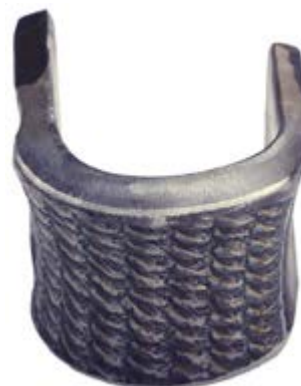
Face Bend: Optimum bead-to-bead tie-in.
