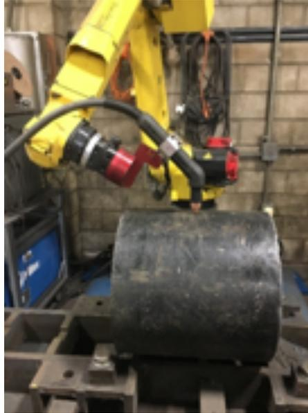
FIG. 3 - ARC cutting robot with PAC torch
