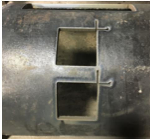
FIG.4 - Pipe section with tensile and Charpy blanks removed
