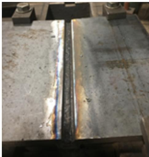
FIG. 2 - Typical filler metal qualification test plate
